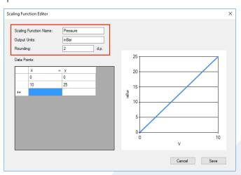
Next, edit the scaling function for the logger. This function is linear between the points specified and the upper and lower points have to remain the upper and lower limits of the logger.
