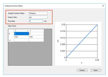
Because the logger reads from 0mA and the sensor output starts at 4mA, the 0 to 4mA part of the function needs to be set to read 0psi. The 20mA point of the function also needs to be re-scaled to 100psi. The edited table looks like this:
