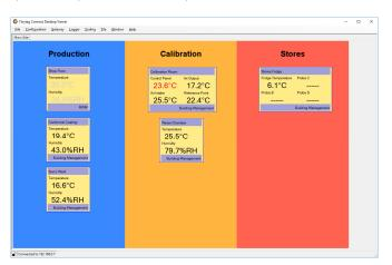
On large sites, or sites with lots of data loggers, multiple windows can be configured to show data clearly. Readings can be scaled, so voltage, current or count loggers being used with third-party sensors can display data in the relevant units.
